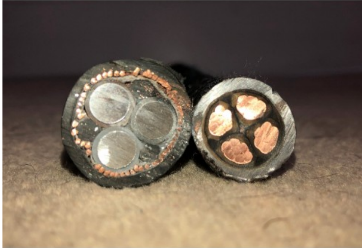
Illustration 4: REC 3-phase cables – CNE & SNE thanks to P. Meenan
